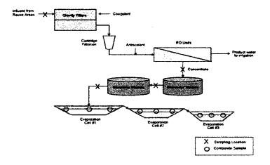
Figure B-I Pilot Selenium Treatment, Reverse Osmosis, and Evaporation Basin System
